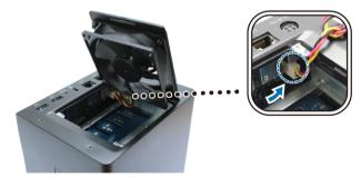
5 Slide one side of the fan into the Synology NAS first then close the fan case.
