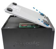
**6** Reconnect the cables you removed in step 1, and then press and hold the power button to turn on your Synology NAS.
