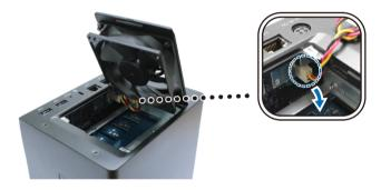
**4** Replace the malfunctioning fan with a new one. Plug the power cord of the new fan into the Synology NAS, as illustrated below.
