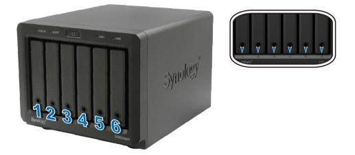
*Note:* If you want to create a RAID volume, we recommend that all installed drives are of the same size to make the best use of drive capacity.
