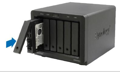
Important: Make sure the drive tray is completely inserted. Otherwise, the drive might not function properly.
