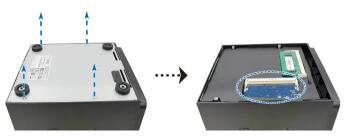
*Important:* When you remove the panel, the sensitive internal components are exposed. Avoid touching anything other than the memory assembly when you remove or add a memory module.
