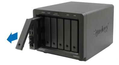
2 Place a drive in the drive tray and tighten the screws provided to secure the drive in place, as illustrated below.
