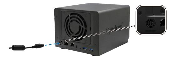
2 Connect at least one LAN cable to one of the LAN ports of the Synology NAS. Connect the other end to your switch, router, or hub.
